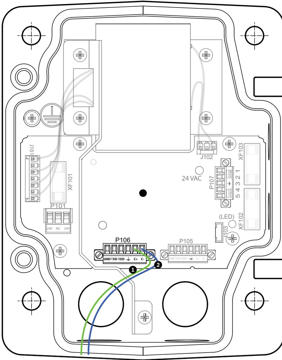
**Figure 10.1:** Detail of P106 Connections
