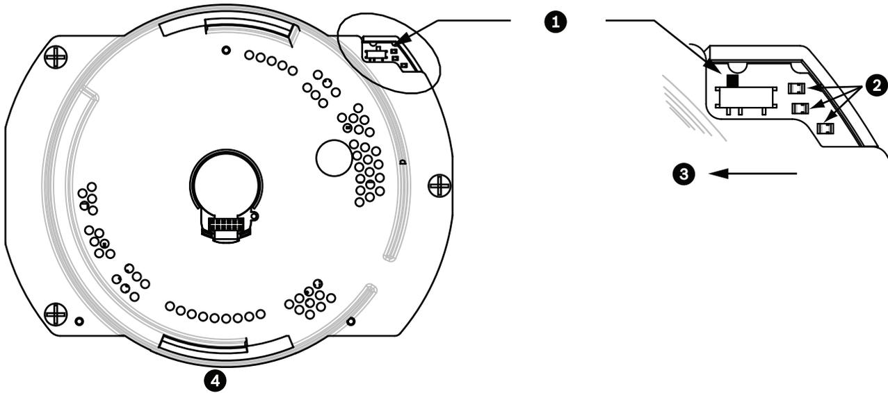
**Figure 10.2:** Position of CPU Switch for RS-232 Operation
