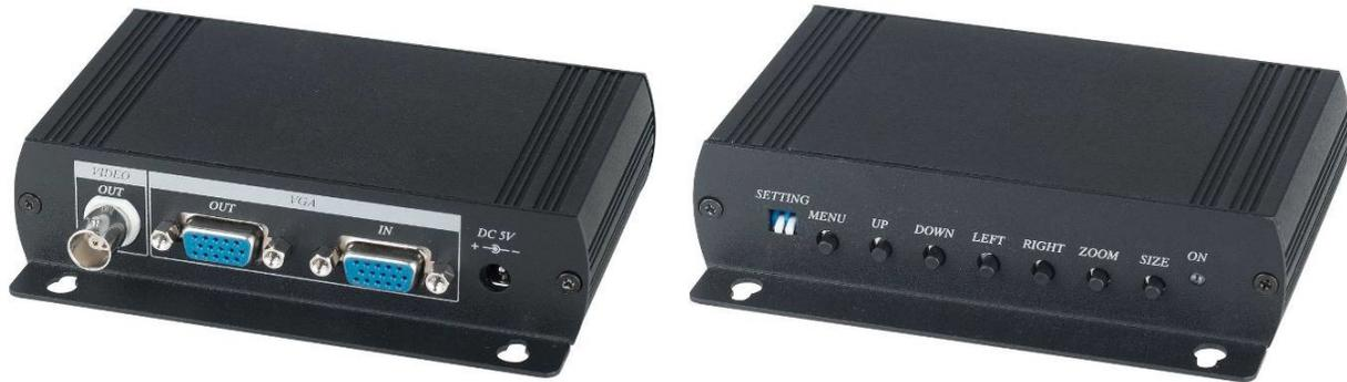
Speco Technologies' VGABNC VGA to BNC converter modifies your VGA signal for viewing on any standard definition TV, projector, or any other device that uses a standard BNC connector. It also features a VGA output that allows for VGA Loop-Through to simultaneously view video on a VGA monitor and CRT TV monitor.
