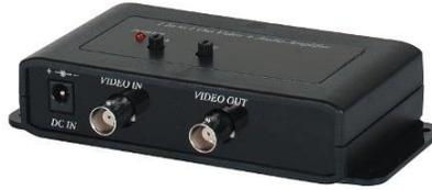
Speco Technologies' VIDAMP amplifier is designed for long-range video transmission of Standard Definition Video up to 3280' over RG59 coaxial cable. The VIDAMP is suitable for long distances, different floors in a building or through different electrical fields.
