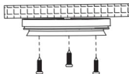
4. Install the camera unit and enclosure to the mounting base and then adjust the dome to obtain an optimum view angle.
