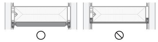
For installation stability, fixed shelf dedicated to 19-inch rack that supports the load of at least 30 kg is recommended.
