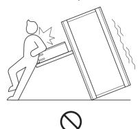
Use a shelf that supports the load of at least 30 kg while it is pulled out, and ensure that there is no deformation on the rail part while in use.
