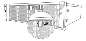
3 Mount a HDD in the HDD bracket and screw it in using the screws provided.
