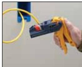
5. Pull trigger completely and remove excess wire prior to releasing trigger.
