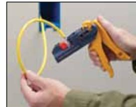
3. Insert jack in JackRapid front first with IDC slots facing blades of JackRapid.
