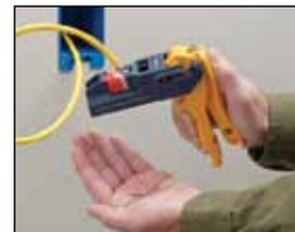
6. Wires will be seated and cut for a solid termination.
