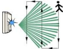
2. Adjust the Microwave Range Adjustment Potentiometer to as low a setting as possible for proper catch performance.
